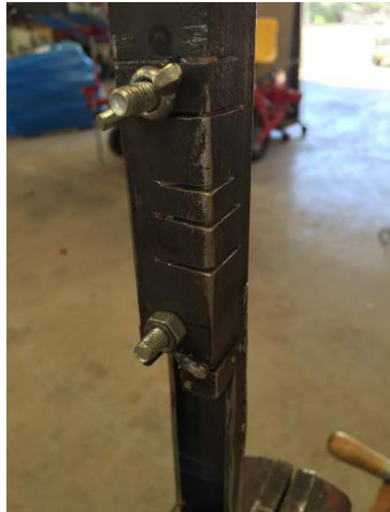
Outer view of final design. Width of strip is determined by the right hand side width of the three slits shown between the screws.
