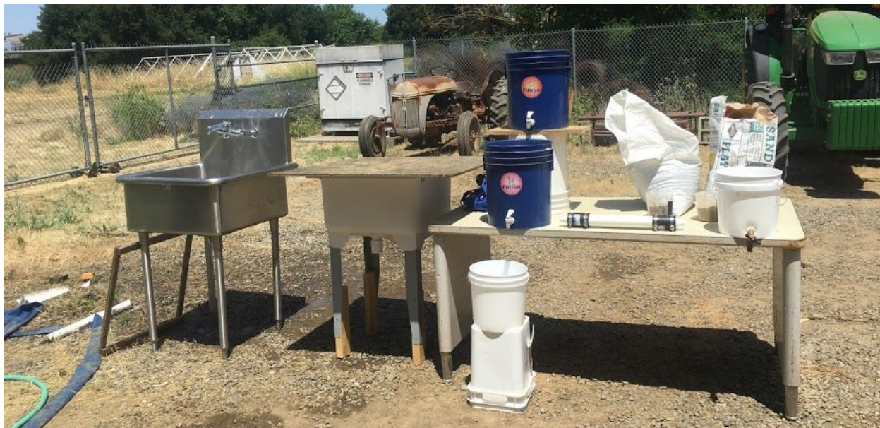
Fig. 7: Prototypes of different parts of our design (Silver sink: sink for crop wash, White sink: sedimentation tank, Blue bucket at the bottom: sand filter, White tube on table: UV chamber, White bucket on the right: Storage tank)
