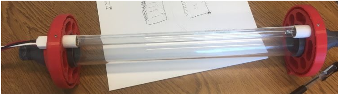
Fig. 5: UV disinfection chamber with 1 UV lamp
