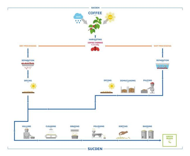
**Figure 6**: Coffee Processing Flowchart. Quality control steps include at harvest, wet processing separation, drying, and sorting.
