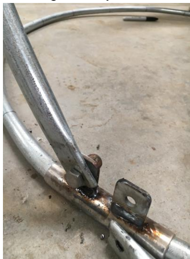
Figure 1. Hinges welded onto connector
