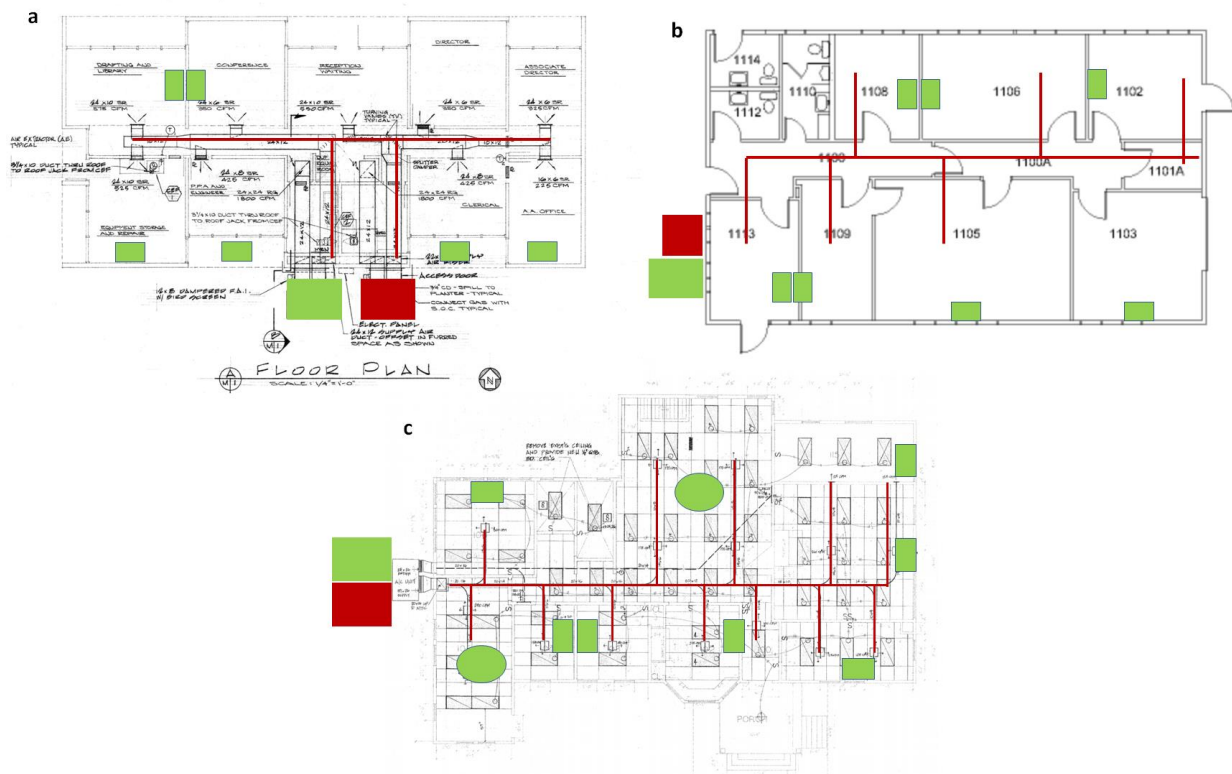
Figure 4. Proposed HRV + VRF design for a) Ag Field Station b) Music Annex and c) University House
