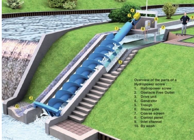
Figure 7: Overview of an Archimedes screw turbine [11]
